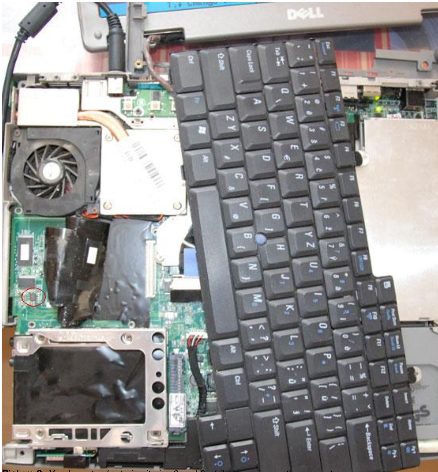
Picture 2. You have to short-circuit pins 3 and 6 while powering on the computer.
